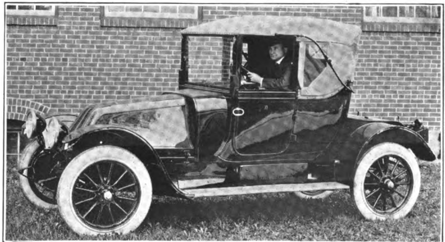
RUNABOUT Body built by Mifflinburg (Pa.) Buggy Co. Mounted on Franklin chassis
